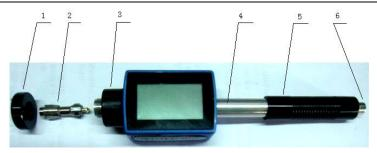
1 Support ring 2 Impact body 3 Coil unit 4 Guide tube
