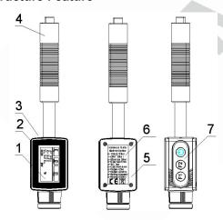
1 LCD display 2 Main unit 3 Socket of USB 4 Impact device
